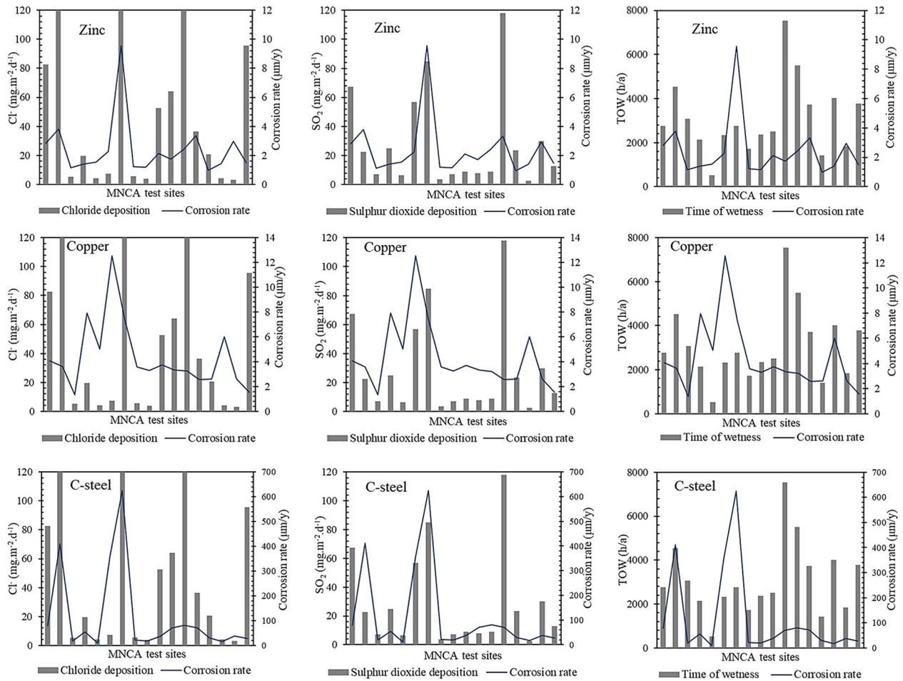
**Figure 12.** Environmental variables and corrosion rates measured in the MNCA in 1990–91 for zinc, copper and carbon steel [3]. The upper limits (y-axis) for Cl<sup>-</sup> were limited in 3 stations (reaching as high as 780 mg.m<sup>-2</sup>.d<sup>-1</sup>) for the sake of better visualisation.
