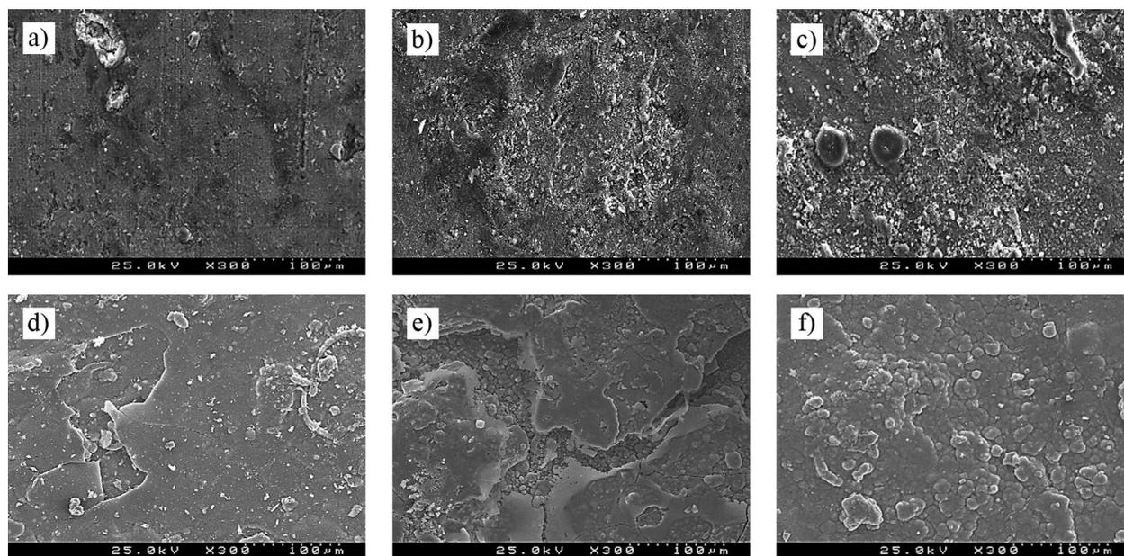
Figure 8. SEM images of zinc (a–c) and cast iron (d–f) surfaces after 1-year exposure in: Fernão de Magalhães Avenue, Coimbra (a,d); Geophysics Institute, Coimbra (b, e); University of Aveiro (c,f).
