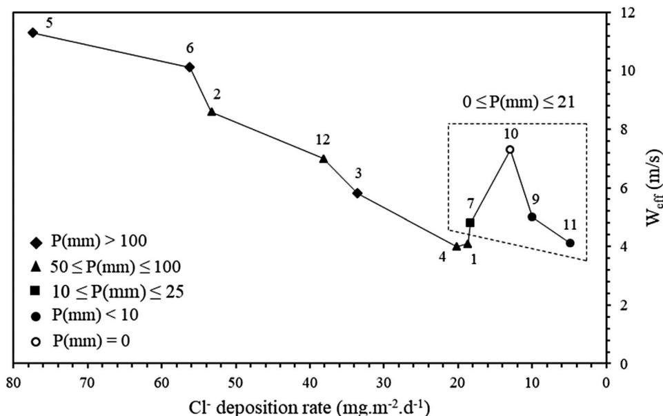
Figure 5. Chloride deposition relationship with effective wind velocity and precipitation.
