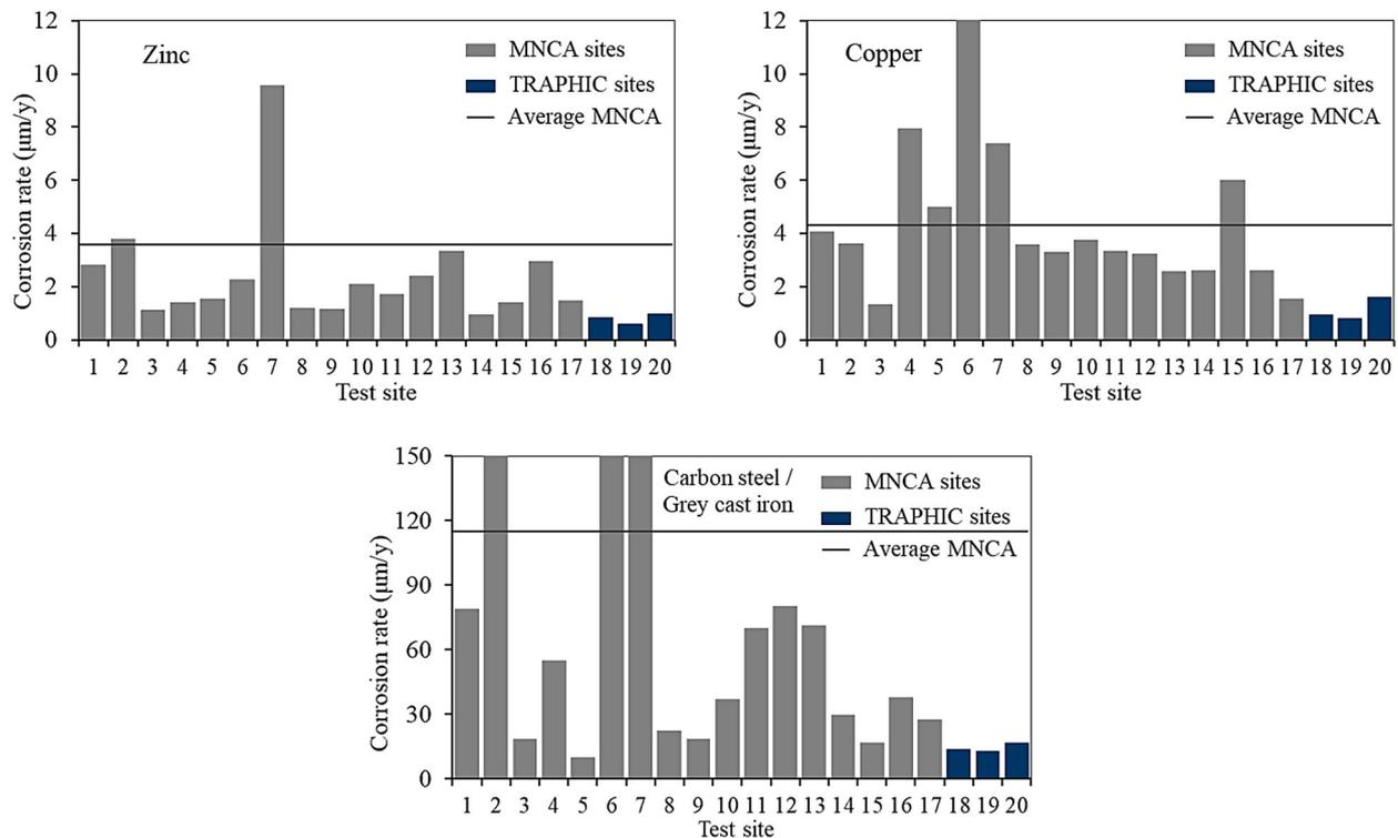
Figure 11. Corrosion rates in 1990–91 (MNCA [3]) and in 2017–18 (TRAPHIC test sites).
