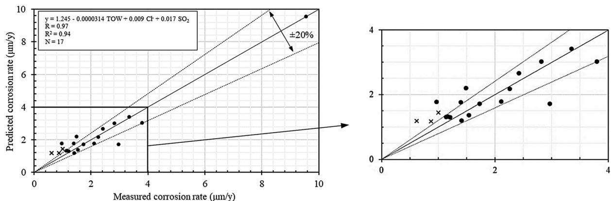
**Figure 13.** Measured vs predicted zinc corrosion rates using the multiple regression expression obtained from MNCA 1990–91 data [3]. TRAPHIC results from 2017 to 2018 are marked as 'x'.
