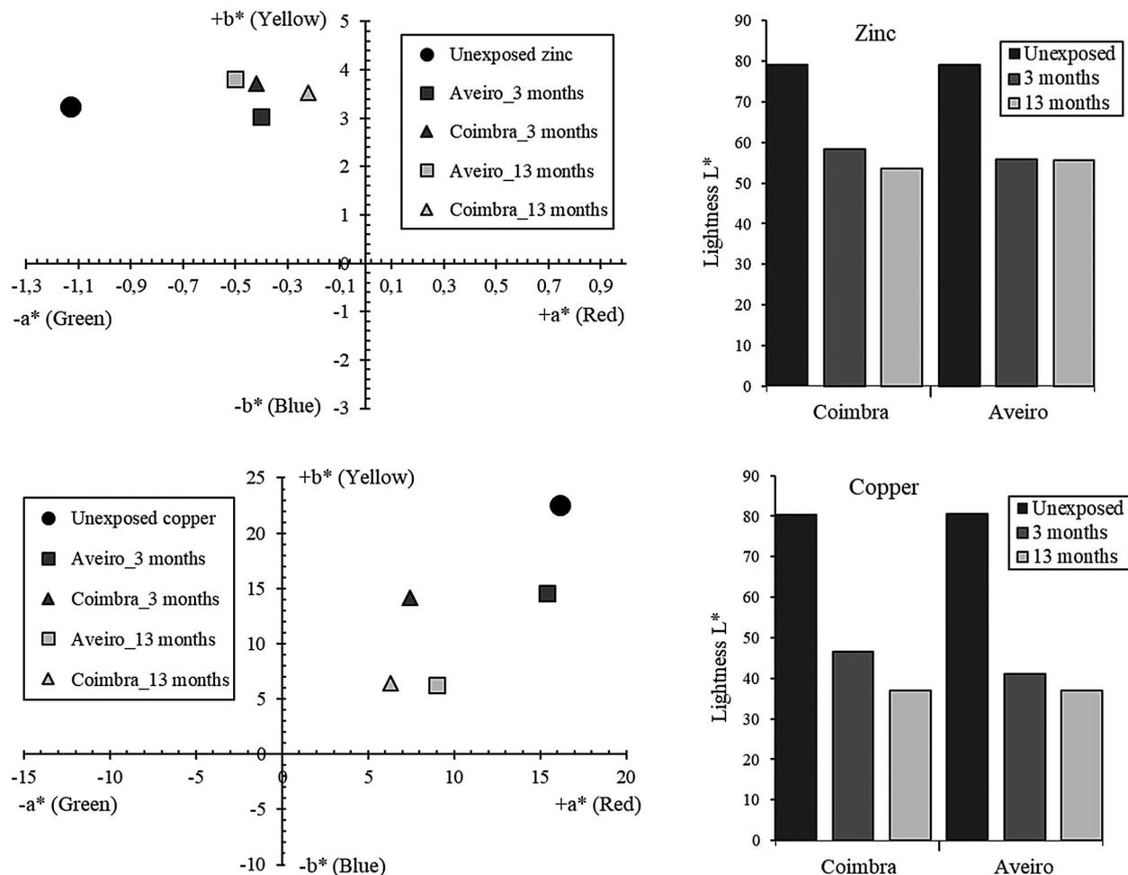
Figure 7. Spectrophotometry results indicating lightness and chromatic changes in copper and zinc.
