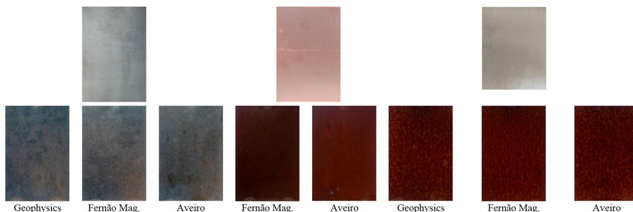
Figure 6. Photographic registration of the unexposed (top) and exposed after 1-year (bottom) samples of zinc (left), copper (centre) and grey cast iron (right). Size of plates is  $10 \times 15 \text{ cm}^2$ .
