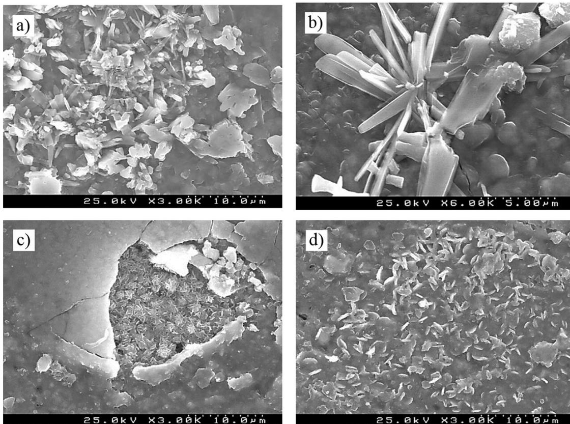
Figure 9. SEM images of copper samples with higher traces of sulphur (a,b) and chlorine (c,d) in total composition.
