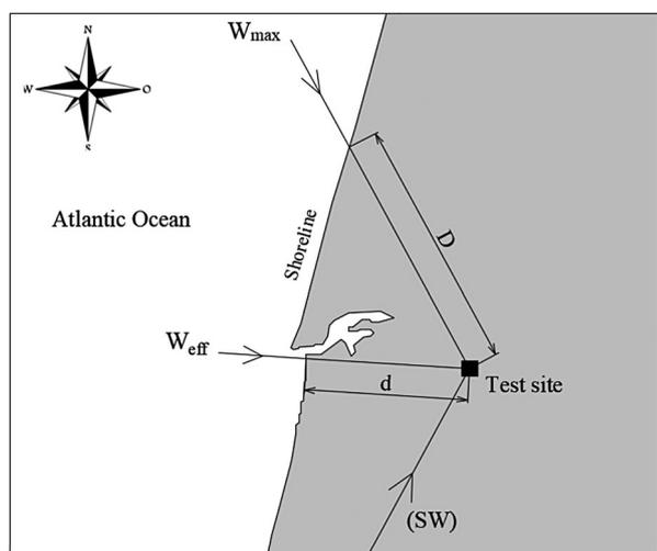
**Figure 4.** Schematic representation of the definition of effective wind (according to distance to shore) as a main factor.
