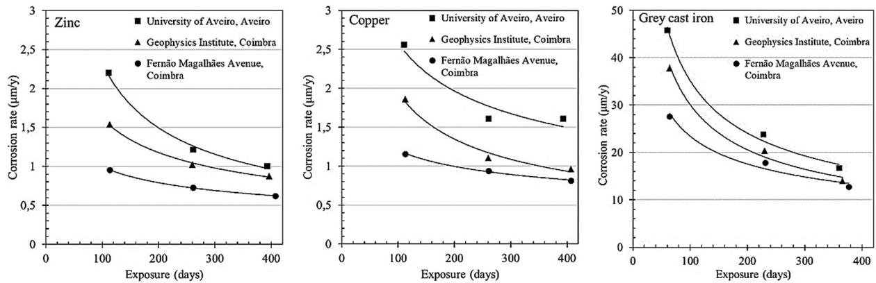
Figure 10. Evolution of the corrosion rates of zinc, copper and grey cast iron during 1 year of exposure in Coimbra and Aveiro.
