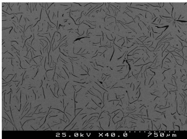
**Figure 2.** Micrograph of the grey cast iron used in this work.
